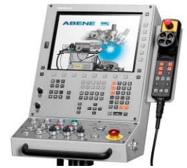
Heidenhain TNC-620 Connections: RJ45 USB port
